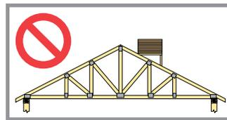
**DON'T** stack materials at or near the midspan of the truss. **Never** exceed stack heights provided in the table (see page 1) unless alternative information is provided by the Building Designer, Truss Designer or Truss Manufacturer.
