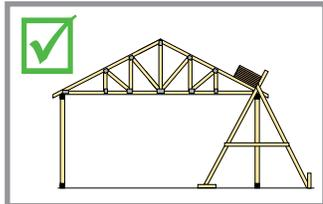
**DO** stack materials along exterior supports or directly over interior supports of properly restrained and braced structures.
