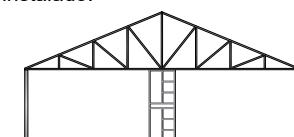
Apply structural sheathing to the top chord as the trusses are being installed.
