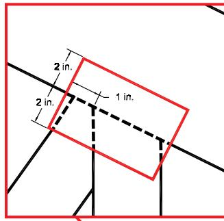
Note: Dimensioned plate locations are sometimes omitted when a plate is to be positioned symmetrically about a joint interface.
