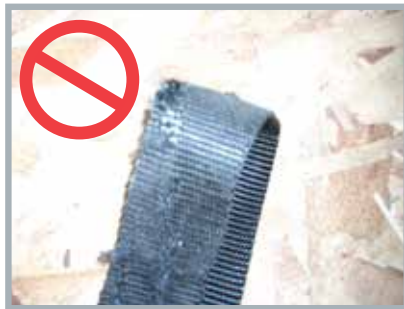
Figure 1: Unacceptable strap and attachment damage
